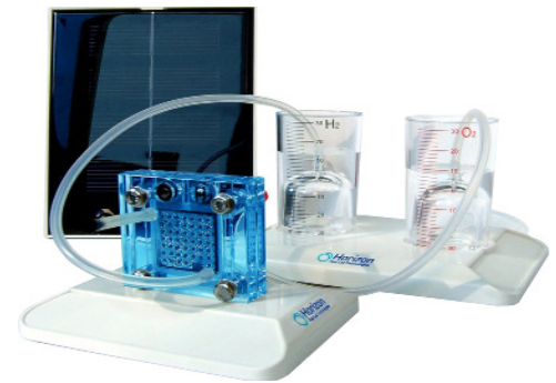
Solar Panel & Fuel Cell
