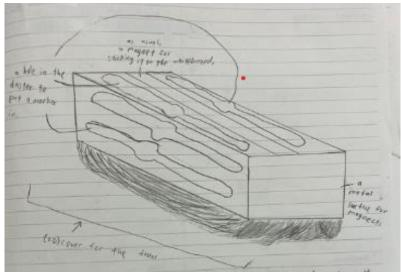
We originally designed the prototype with a horizontal plastic bar over the slot for markers. However, we discovered that it made rattling sounds whenever teachers wiped the whiteboard as the markers could freely move about within the space.
