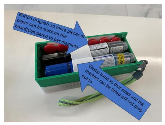
In our final prototype design, we removed the horizontal bar and used elastic bands to secure the markers in place to ensure that they would not fall out easily and would not make rattling noises (see section IV "3-D printed prototype with explanation of the various design functions"). The elastic bands also cater to different teachers' preferences, as they will be able to accommodate 2 to 3 markers of different sizes, big and small.
